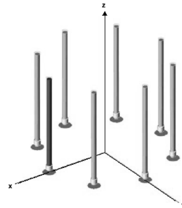
Fig.18. Radiation pattern eight-element plasma antenna array
