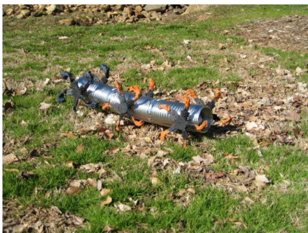
Fig.13 Initial FRESE IV prototype on smooth terrain.
