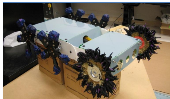
Fig.5 Initial prototype, FRESE I. Note front "tentacle-wheels" and rear whegs.
