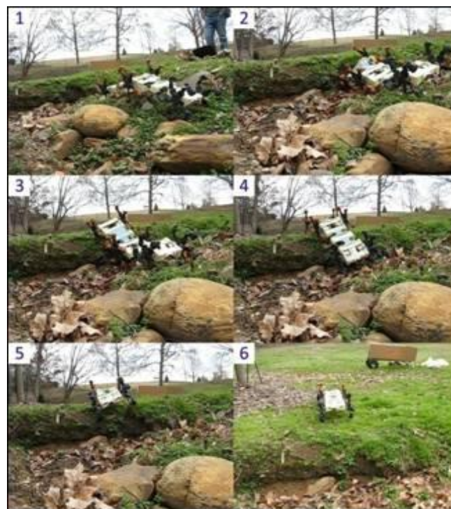
Fig.12 FRESE III climbing a rocky slope.
