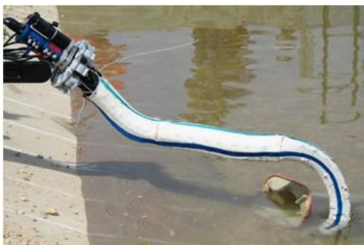
Fig.2 Octarm continuum manipulator - hook mode.
