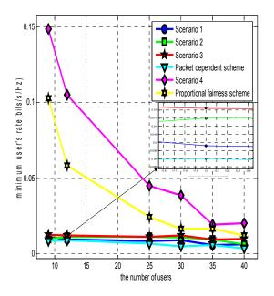
Fig.11 Minimum user's rate versus the number of users
