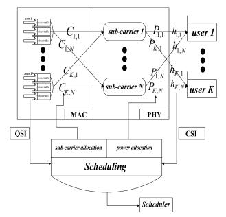
Fig.1 the block diagram of multi-user OFDM system
